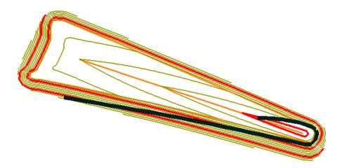
The result is a 3D MicroStation linestring that follows the defined longitudinal slope, traversing the surface selected. Vertices are created for the linestring at each crossing of a triangle. You can now import the graphic as a horizontal and vertical alignment using File > Import > Geometry from Graphics, refine the alignments as necessary, and use them in Roadway Designer to create the access road.
