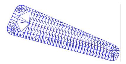
Here, you'll notice that there are triangles cutting across the corners, causing some erroneous contours. See the process for **Place Features** in this chapter for a suggestion on how to combat this situation and further enhance the surface.
