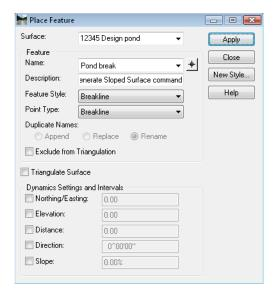
In this example, a breakline is added to enhance the triangulation of a sloped bottom pond. Notice how the contours do not follow the shape of the pond bottom in the corners.
