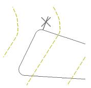
In this case, multiple points are checked along the element to see where the slope intercepts. The endpoints of these lines could be joined with a linestring and loaded as a feature for the toe of slope, or you can now use **Generate Sloped Surface** to create the features after identifying the desired slope with the **Project Line to Surface** command.
