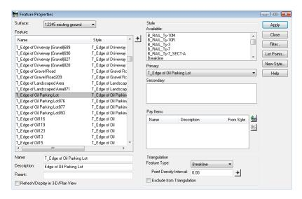
The Feature Properties command (Surface > Feature > Feature Properties) provides a list of all of the features contained in the surface and the style assigned to each feature. Use this dialog box for a variety of functions including:
