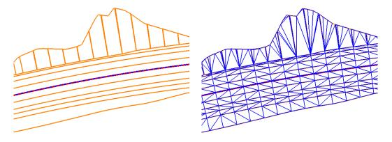
Notice in this case, you may need to add additional features to "catch" each of the vertices in the new toe of slope.
