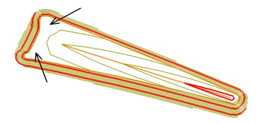
Displaying the triangles shows why; in the corners the triangles have all three points touching the edge of the pond bottom, with nothing projecting to the drain line in the middle of the pond. Breaklines can help resolve this issue, resulting in a better surface model.
